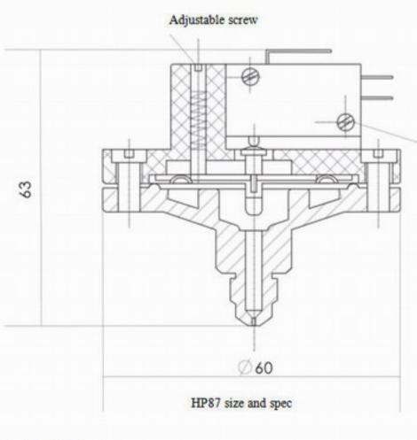
Don't touch the sealed screw, which has been adjusted and sealed in factory.
